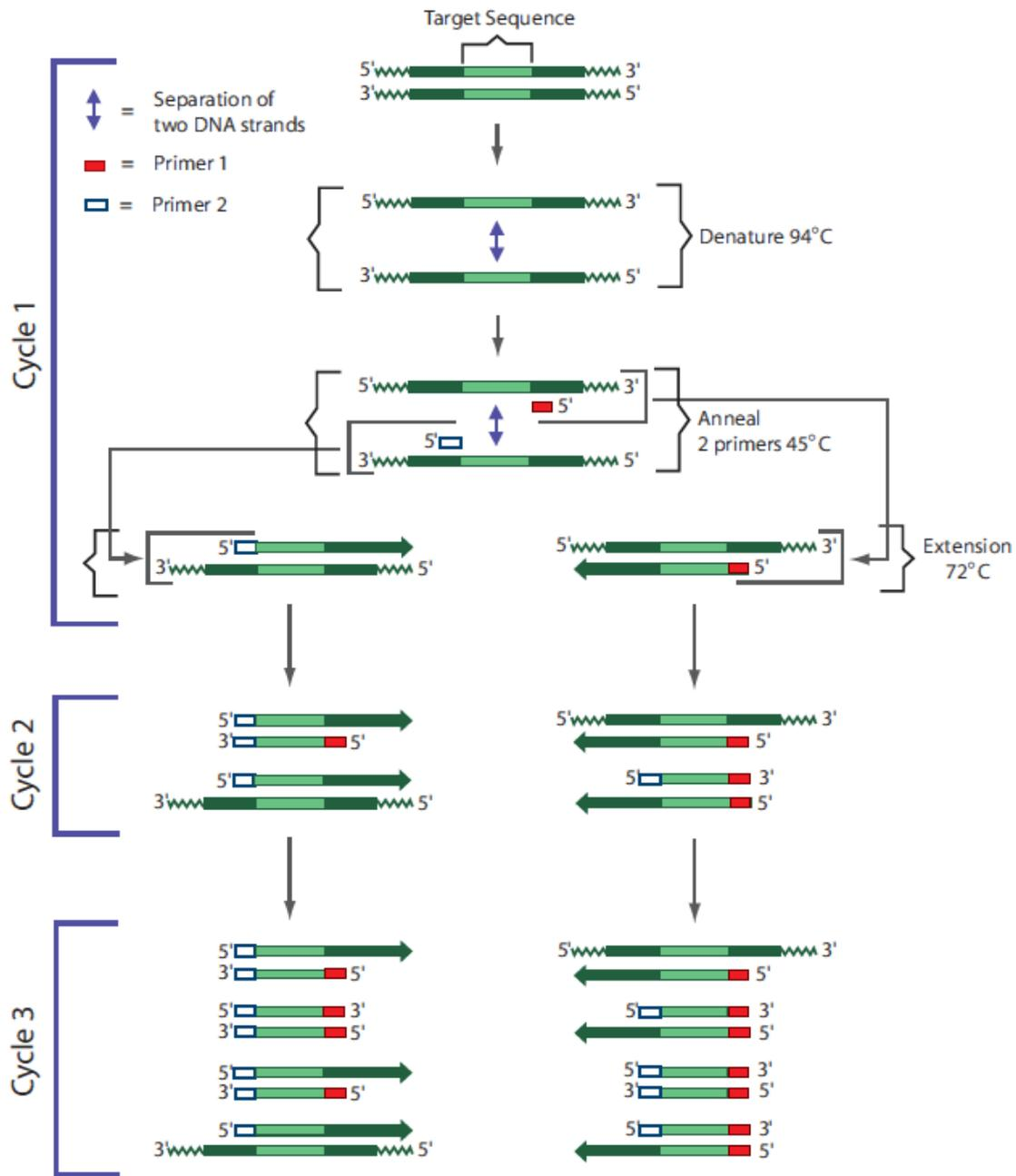
These three steps, denaturation-annealing-extension, constitute a PCR cycle. This process is repeated for 20-40 cycles by amplifying the object sequence exponentially. The PCR is performed on a **thermocycler**, an instrument that is programmed for rapid heating, cooling and maintenance of the samples for several times. The amplified product is then detected by removal of the reaction mixture by agarose gel electrophoresis.
