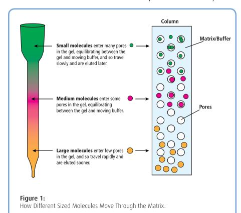
Filling the chromatography column with matrix is referred to as "packing". The packed matrix is called the "bed" and the volume it occupies is termed the "bed volume". It is very important not to allow the bed to run dry. Otherwise, cracks and fissures develop and the matrix has to be removed and repacked.
